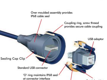
Panel gasket maintains IP68 seal to panel
